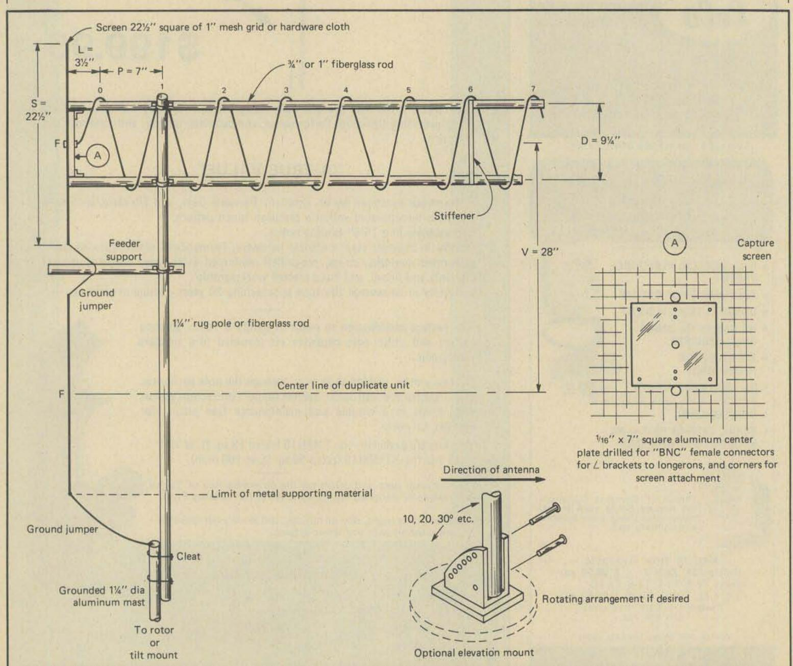
Fig. 1- Mechanical diagram for the helix antenna. It should be noted that it bears no relation to the other double helix by Watson and Crick.
